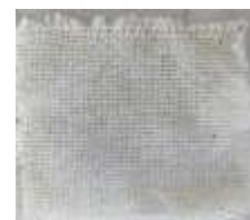
(G) Washed with distilled water (97mL) + detergent (1mL) + protease (2mL)
